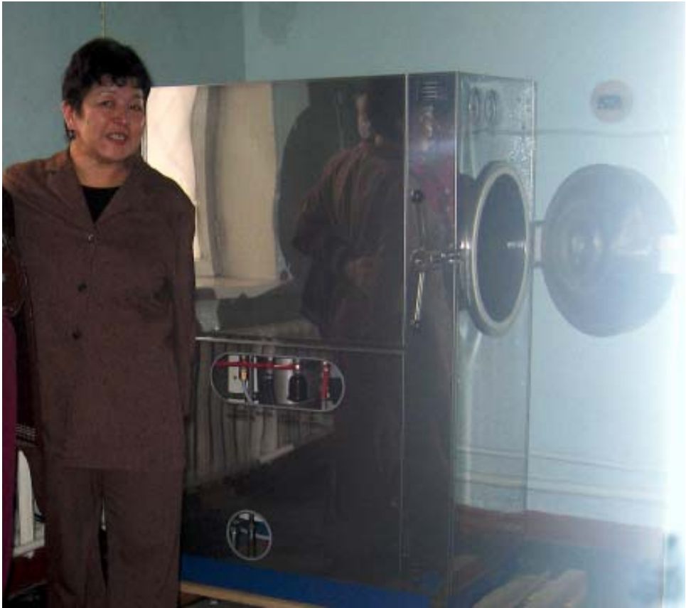
Fig. 53. An autoclave. The steam-pressure vessel, used for sterilization.
