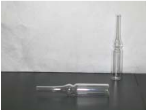
Fig. 54a. Glass ampules used to store mycelium in a liquid nitrogen refrigerator.
